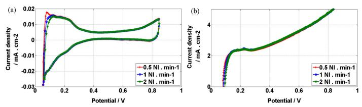
Fig. 2. Example of hydrogen and nitrogen flow rate effects on the CV (a) and LSV (b) diagrams (case: Tests 1, 2, 3).
