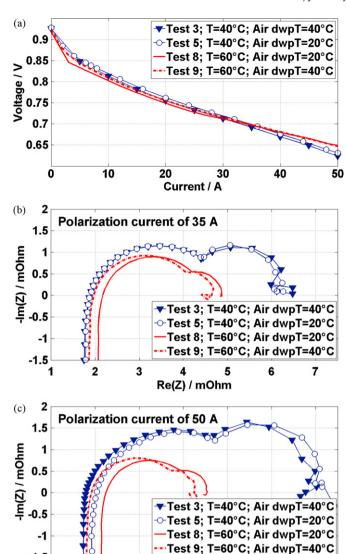
**Fig. 3.** Effects of air dew point temperature (Air dwpT) on the FC performances. (a) Polarization curves recorded for different air dew points (FSA = 2 and FSC = 3 for operating temperature (T) = 40 °C) (FSA = 2 and FSC = 5 for T = 60 °C). (b) Impedance spectra at 35 A for different air dew points (FSA = 2 and FSC = 3 for T = 40 °C) (FSA = 2 and FSC = 5 for T = 60 °C) at 35 A. (c) Impedance spectra at 50 A for different air dew points (FSA = 2 and FSC = 3 for T = 60 °C) at 35 A.
